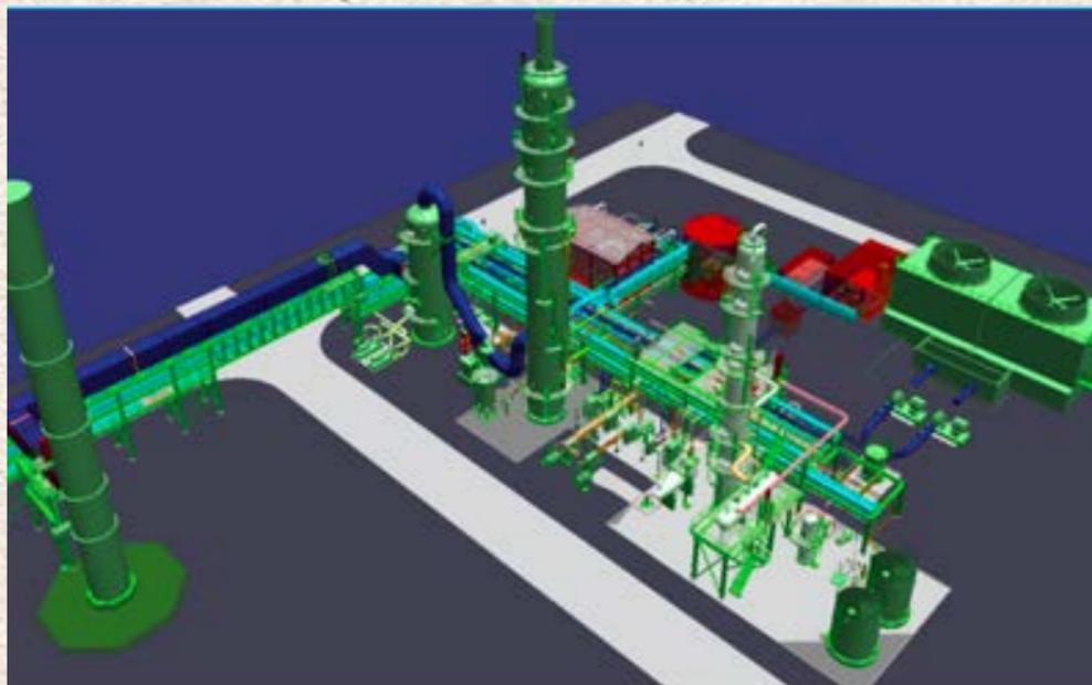
Figure 10. Carbon Dioxide Recovery 3D View
